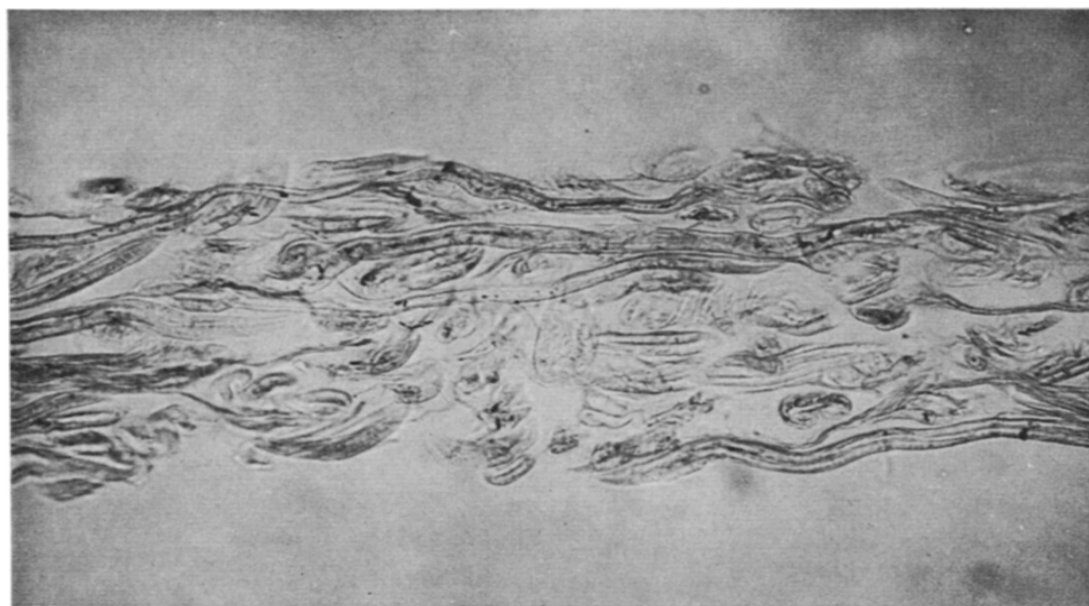
Fig. 3. Cross-section (10 \mu thick, wax-embedded, wax removed) of Whatman No. 1 filter paper. Note some shrinkage of fibre due to embedding. Mag. (section to photo) \times 200 .
